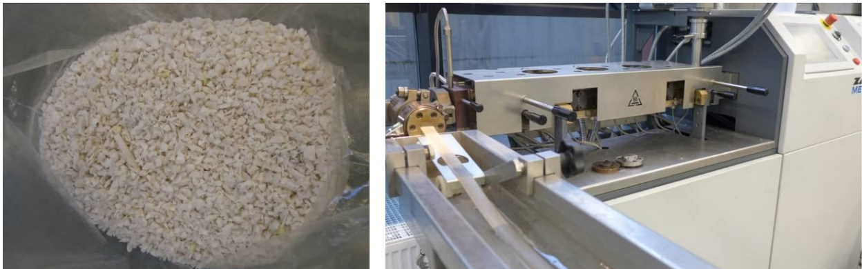
Fig.1. An example of a plastic sample after the comminution process and view of technological line section for recycled plastics
